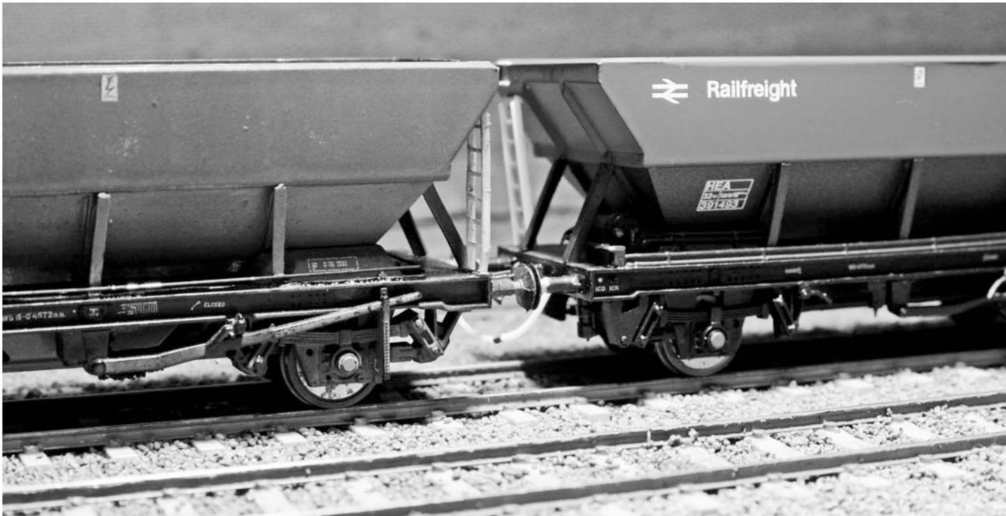
I think it best to begin by defining what “working” means. Ok there is no air or vac braking system, the brakes on the vehicles don’t actually come on and off but what I mean is these brake pipes connect up.
